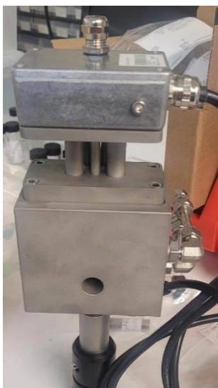
Fig. 1: Image of 'Mjolnir' the high temperature in situ cell (left) and a temperature calibration curve showing the variation in the temperature between the cell and a model pellet.
